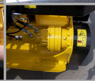
Trasmissione idraulica del pick-up Transmission hydraulique du pick-up Pick-up hydraulic transmission Hydraulischer Antrieb vom Pick-up Transmisión hidráulica del pick-up
