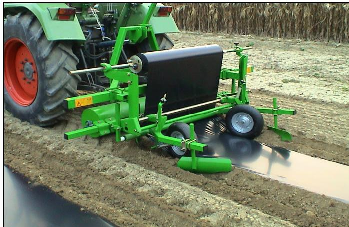
The **MULCHING MACHINE** is laying down plastic and nylon roller of different widths. It can be equipped with or without front roller and with rear rubber wheels. All parts of the machine are adjustable according to the size of the roller 1,40 m or 1,90 m wide models are available.
